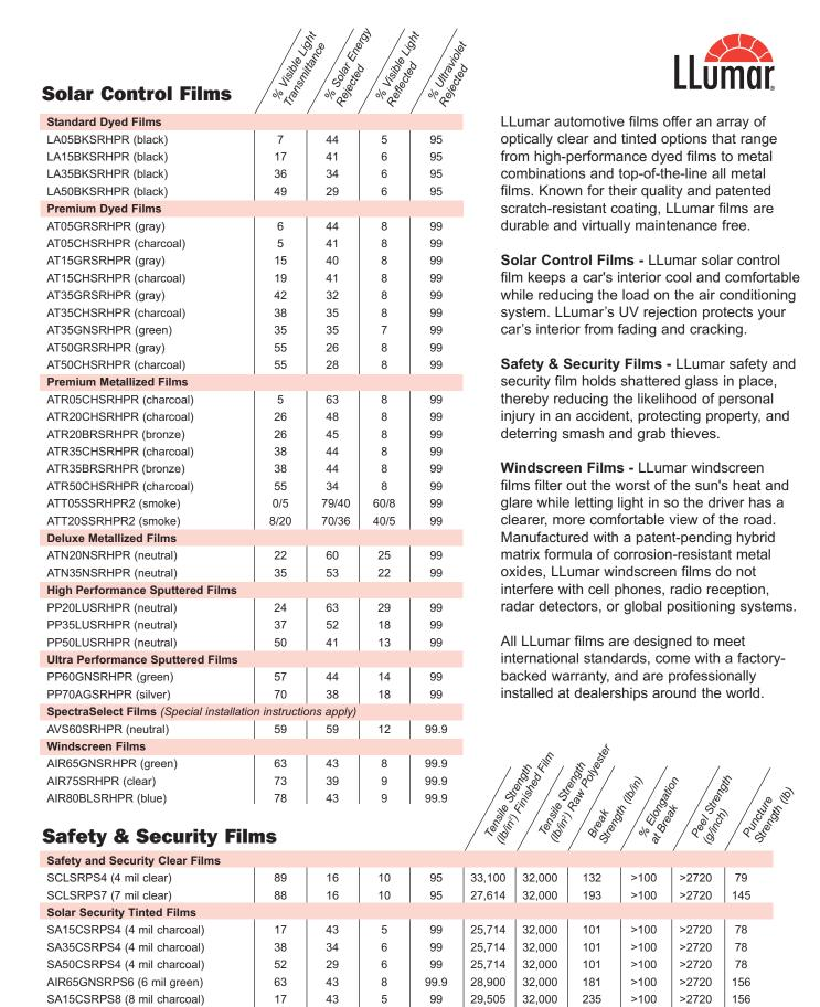
Typical solar properties with film mounted to 3mm clear glass. All values averaged from routinely accumulated quality control data.
